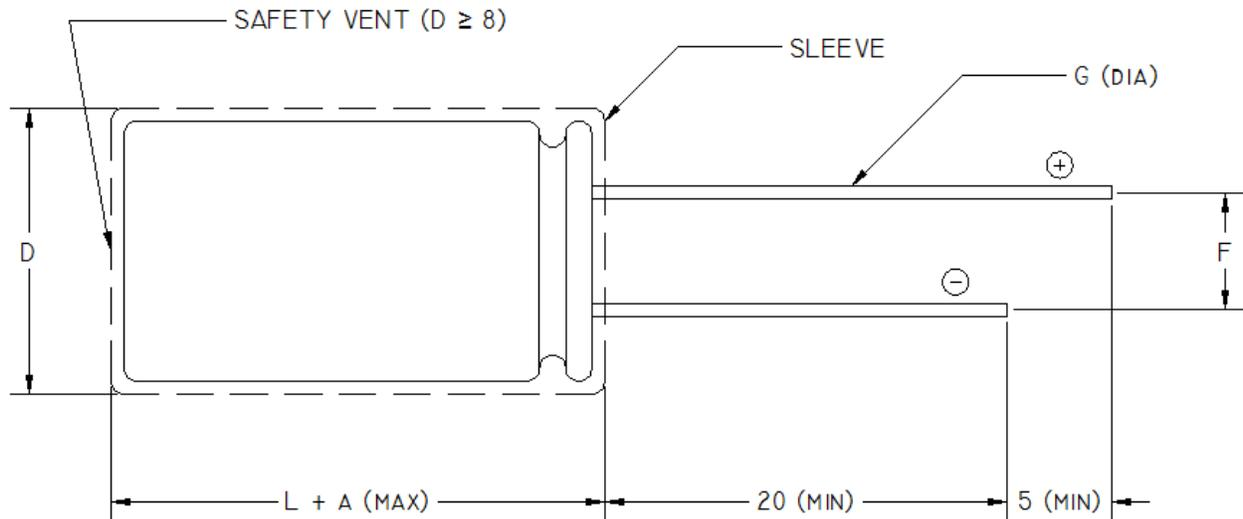
Dimensions are in millimeters (mm)
